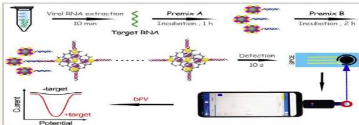
Fig. 8 Systematic process for COVID-19 detection by means of Electro-chemical biosensor (a). premix A and B preparation ; (B) procedure of Electro-chemical method using smart-phone [14]
